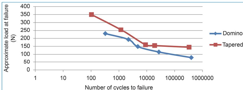
**Figure 4.** The load to number-of-cycles-at-failure curve.
