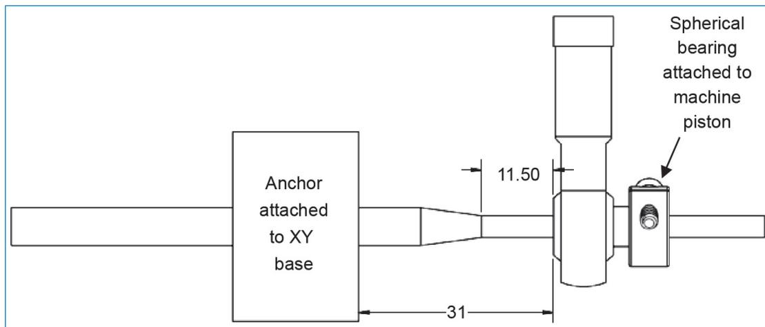
Figure 2. The tapered titanium rod construct (side view).
