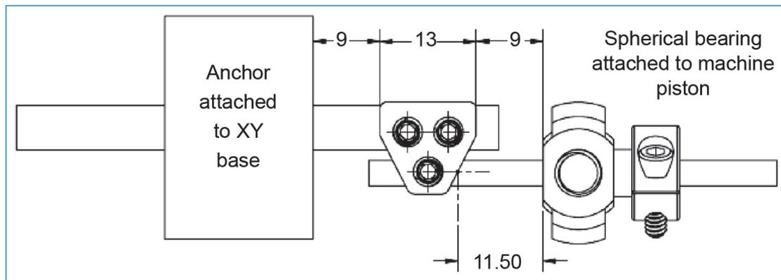
Figure 1. The domino connected rod construct (top view).
